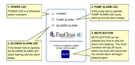
Normally when the system is operating correctly, only the green POWER LED is lit to indicate that power is available.
